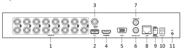
\*: The rear panel of iDS-7204HQHI-M1/S provides 4 video input interfaces. The rear panel of iDS-7208HQHI-M1/S provides 8 video input interfaces.
