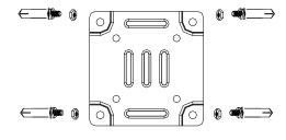
4  $% \sub{4}{3}$  Install the bracket to the pre-installed plate
