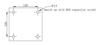
③ Fix the pre-installed plate
