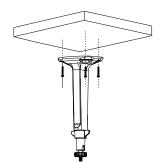
③ Adjust the monitoring angle through nut and universal joint
